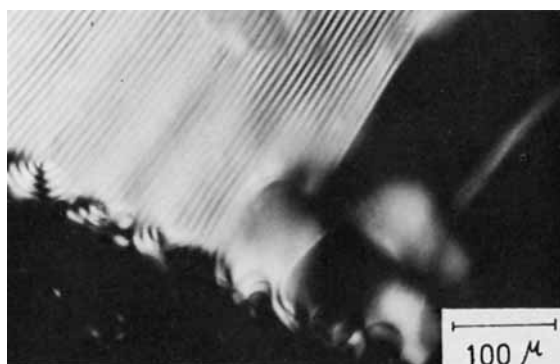
Fig. 20. Polarizing micrographs of PGA-PEG900-DMF [PGA/PEG = 70/30, (PGA + PEG)/(PGA + PEG + DMF) \times 100 = 18.5%].
